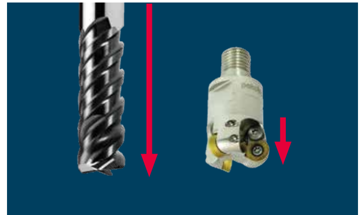
HPC和可转位刀片刀具的对比
